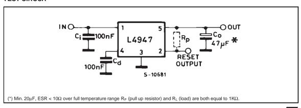
**ELECTRICAL CHARACTERISTICS** (refer to the test circuit,  $V_i = 14.4V$ ,  $C_o = 47\mu F$ , ESR <  $10\Omega$ ,  $R_p = 1K\Omega$ ,  $R_L = 1K\Omega$ ,  $-40^{\circ}C \le T_J \le 125^{\circ}C$ , unless otherwise specified)
