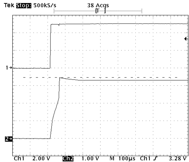
Figure 9 - Input voltage transient response, V_{IN} from 0V to 5V, C_{OUT}=10\mu\text{F} . Ch2 Peak: 3.48V Ch1: 5V input voltage, 2V/div Ch2: 3.3V output voltage, 1V/div
