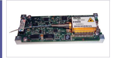
The Oclaro LambdaFLEX<sup>TM</sup> iTLA is a high performance continuous wave (CW) tunable laser source for use in the L-band window covering 1568nm to 1607nm. Based on the OIF iTLA standard, the laser and control electronics are pre-mounted on a dedicated circuit board for easy production installation. The iTLA features shuttered tuning, trace tone and FM dither circuitry. Comprehensive control and system reporting is provided over the RS232 interface.
