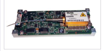
The Oclaro LambdaFLEX<sup>™</sup> iTLA is a high performance continuous wave (CW) tunable laser source for use in the C-band window covering 1528nm to 1563nm. Based on the OIF iTLA standard, the laser and control electronics are pre-mounted on a dedicated circuit board for easy production installation. The iTLA features shuttered tuning, trace tone and FM dither circuitry. Comprehensive control and system reporting is provided over the RS232 interface.
