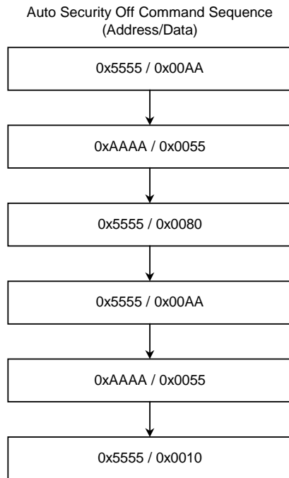
Figure 3.33 Auto Security Off Operation
