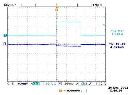
W83310S-R V<sub>OUT</sub> offset with a 1.5A/10ms sinking pulse current.
