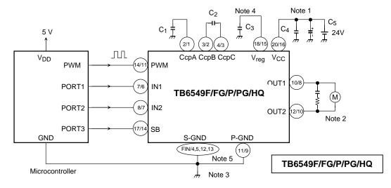
TB6549F/FG: Pins 1, 5, 6, 9, 13, 15, 16, and 19 are not connected. TB6549HQ: Pins 4, 6, 8, 9, 13, 17, 18, 20, 21, 22 are not connected.
