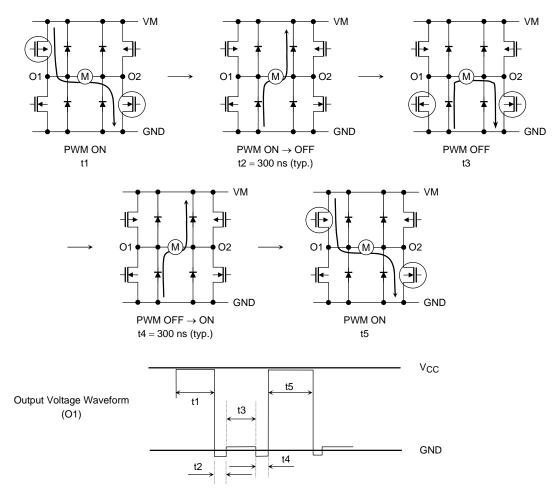
Note: Be sure to set the PWM pin to high if the PWM control function is not used.
