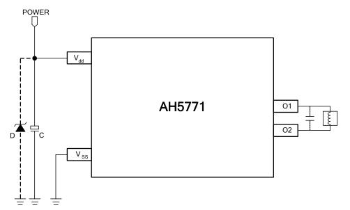
Notes: 3. D (Zenor Diode) and Capacitor C are for power stabilization, D is recommended to be 18Vz (option), C is recommended to 0.1µF ~1µF (E-Cap).
