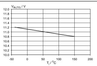
Fig.31. Typical short circuit load threshold voltage.  $V_{BL(TO)} = f(T_j)$ ; condition  $V_{BG} = 16 \text{ V}$
