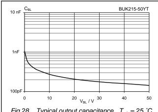
Fig.28. Typical output capacitance.  $T_{mb} = 25$  °C  $C_{bl} = f(V_{BL})$ ; conditions f = 1 MHz,  $V_{lG} = 0$  V
