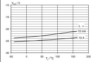
Fig.24. Typical negative load clamping voltage.  $V_{LG} = f(T_j)$ ; parameter  $I_L$ ; condition  $V_{IG} = 0$ V
