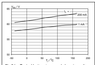
Fig.21. Typical battery to ground clamping voltage.  $V_{BG} = f(T_j)$ ; parameter  $I_G$
