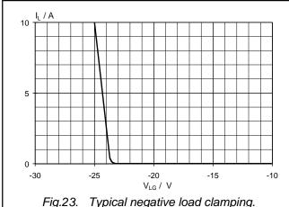
Fig.23. Typical negative load clamping.  $I_L = f(V_{LG})$ ; conditions  $V_{IG} = 0V$ ,  $T_j = 25$ °C
