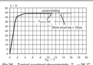
Fig.26. Typical overload characteristic,  $T_{mb} = 25$  °C.  $I_L = f(V_{BL})$ ; condition  $V_{BG} = 16$  V; parameter  $t_p$
