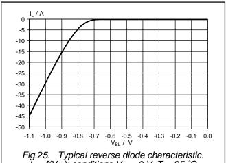
$I_L = f(V_{BL})$ ; conditions  $V_{IG} = 0$  V,  $T_i = 25$  °C
