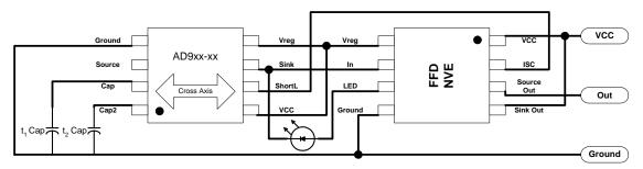
Note: For current-sinking applications, connect "Source Out" to Ground; use "Sink Out" pin as output.
