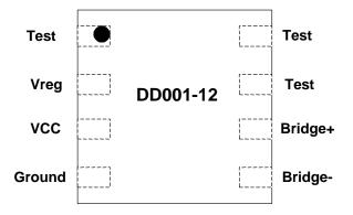
Note: Bridge + and Bridge - should be connected only to the sensor element outputs for ESD and loading reasons. Vreg can supply up to 10 mA at 3.3V (330 $\Omega$  load). Also, all pins labeled "Test" must be floating, *i.e.*, not connected to each other or any other circuit node.
