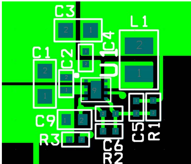
Figure 2. AOZ1605 (DFN-8) PCB Layout
