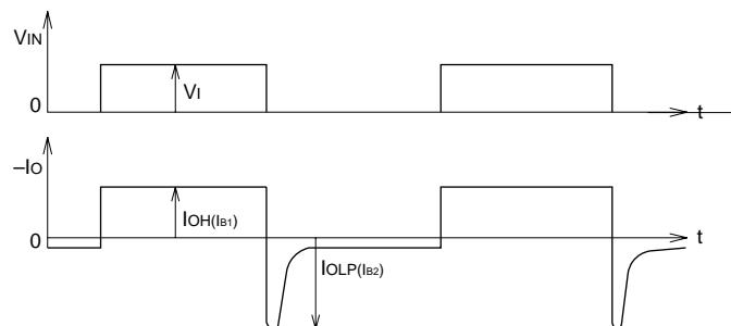
**Note:**  $I_{OH}$  and  $I_{OLP}$  correspond to base forward current  $I_{B1}$  and base reverse current  $I_{B2}$  of the transistor module to be driven respectively.
