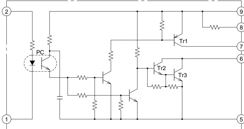
**HYBRID IC FOR DRIVING TRANSISTOR MODULES****ABSOLUTE MAXIMUM RATINGS** ( $T_a = -20 \sim +70^\circ\text{C}$ , unless otherwise noted)
