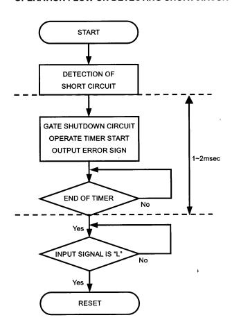
(\*) "L" output voltage with protection circuit operating is about - |V<sub>FF</sub>| + 2V.
