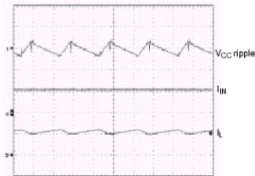
Figure 25. Boost Input Voltage and Current Ripple Waveforms
