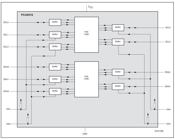
Figure 2. Block Diagram: PCA9516
