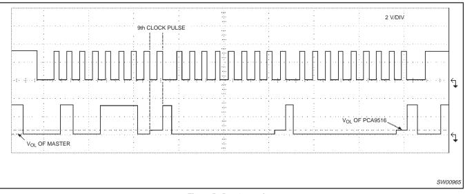
Figure 5. Bus 0 waveform
