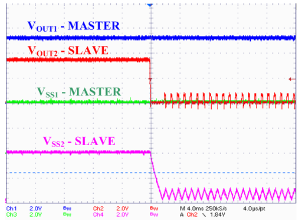
Figure 57. Master Voltage – End of Augmented OLM
