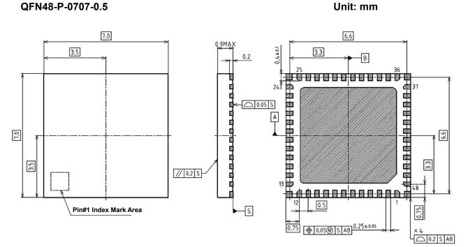
Backside heatsink: 5.4 mm  $\times$  5.4 mm
