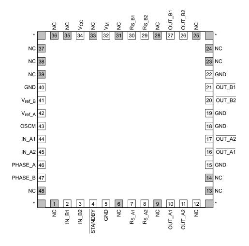
\*Mark PAD: It must be connected to GND
