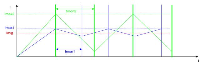
Conclusion: In most cases the coil is driven in a combination of both ways. A tradeoff has to be made between EMI behaviour and maximum allowed LED current. By varying these parameters, an optimum can be found for virtually every application.
