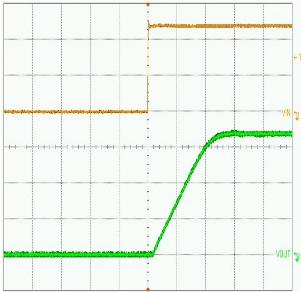
( V_{in} = 12\text{ V} , I_{LOAD} = 10\text{ mA} , L = 5\text{ }\mu\text{H} , C_{OUT} = 100\text{ }\mu\text{F} ) Upper trace: Input voltage, 5 V/div Lower trace: Output voltage, 1 V/div Time base: 500 \mu\text{s}/\text{div}
