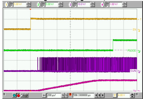
Top: EN2, CH2 Enable Signal, (5V/div) Middle 1: PGOOD2, CH2 Power Good Signal, (5V/div) Middle 2: SWN2, CH2 Switching Node Voltage, (10V/div) Bottom: V_{O2} , CH2 Output Voltage, (1V/div) Time: 200µs/div
