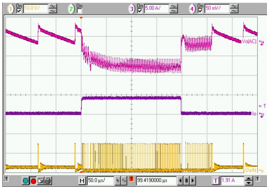
Top: Vo1, CH1 Output Voltage Ripple, (50mV/div) Middle: Io1, CH1 Output Current, (5A/div) Bottom: SWN1, CH1 Switching Node Voltage, (10V/div) Time: 50µs/div
