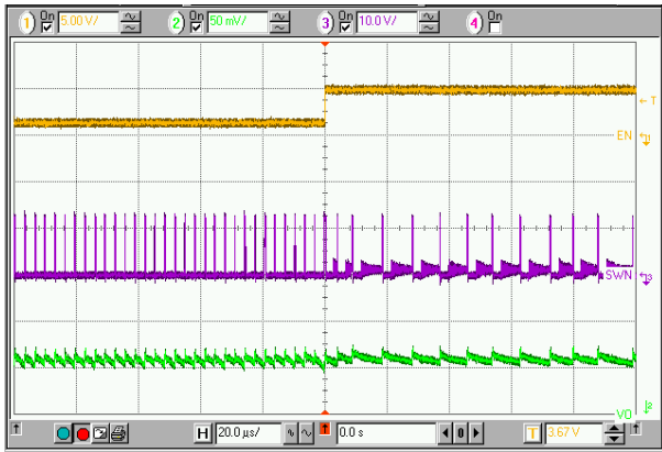
Top to Bottom: SWN_Slave, SWN, V O Figure 11. On Line Mode Change (CCM → DCM)
