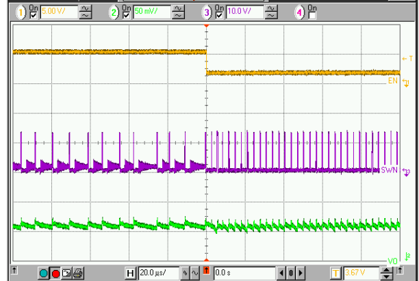
Top to Bottom: EN, SWN, V O Figure 12. On Line Mode Change (DCM → CCM)
