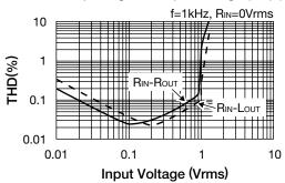
5. THD of output signal – Input voltage (QSrround f=1kHz, The signals that are inputted in Lin and Rin are out out of phase and same amplitude.
