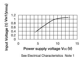
7. Input voltage (2) - Power supply voltage (QSrround)
