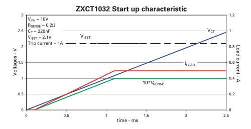
2 The output voltage also increases due to the load current powering up the load and charging any capacitance. After the initial soft start (load current stabilizing) the timing capacitor charges up to 4V and the device enters its normal mode of operation. The external MOSFET will be now fully enhanced minimizing any serial voltage drop.
