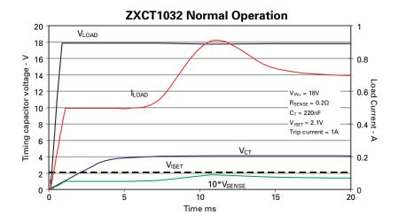
The ZXCT1032 has now entered its over-current detector mode; it is effectively "transparent" to the load until the current monitor output exceeds the trip point.
