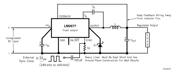
FIGURE 1. Basic circuit for fixed output voltage applications.
