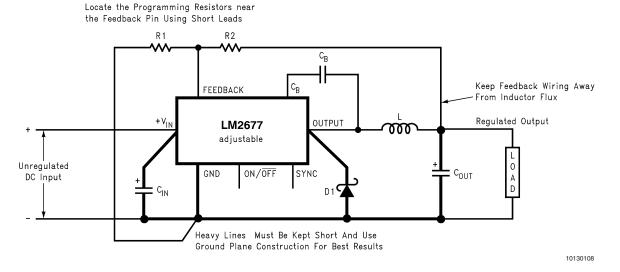
FIGURE 2. Basic circuit for adjustable output voltage applications
