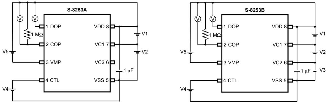
**Figure 5 Test Circuit 1**
