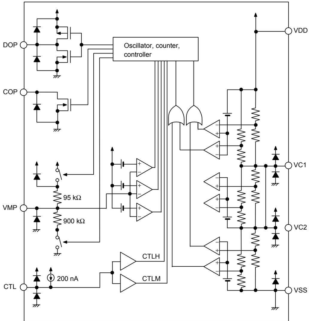
**Remark** All diodes shown in figure are parasitic diodes.
