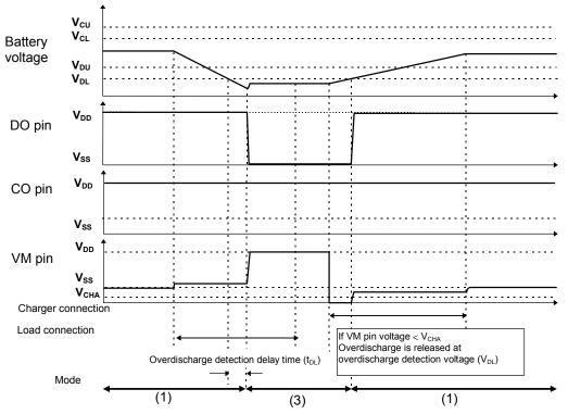
Note: (1) Normal mode, (2) Overcharge mode, (3) Overdischarge mode, (4) Overcurrent mode The charger is assumed to charge with constant current.
