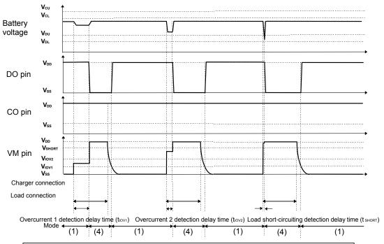
Note: (1) Normal mode, (2) Overcharge mode, (3) Overdischarge mode, (4) Overcurrent mode The charger is assumed to charge with constant current.
