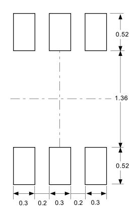
Caution Making the wire pattern under the package is possible. However, note that the package may be upraised due to the thickness made by the silk screen printing and of a solder resist on the pattern because this package does not have the standoff.
