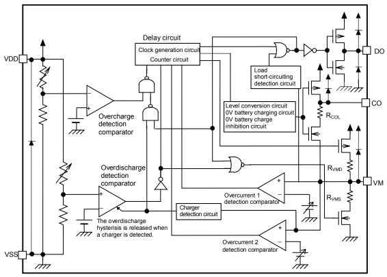
Remark The diodes in the IC are parasitic diodes.
