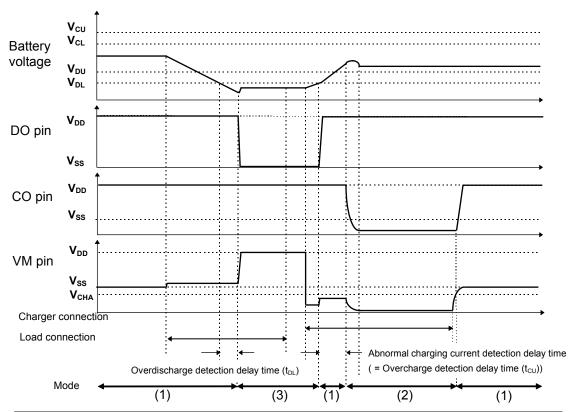
Note: (1) Normal mode, (2) Overcharge mode, (3) Overdischarge mode, (4) Overcurrent mode The charger is assumed to charge with constant current.
