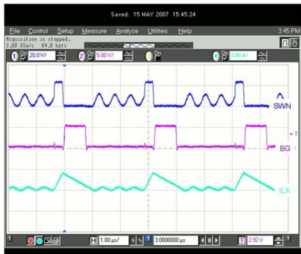
Figure 23. Switcher Operation – DCM Mode
