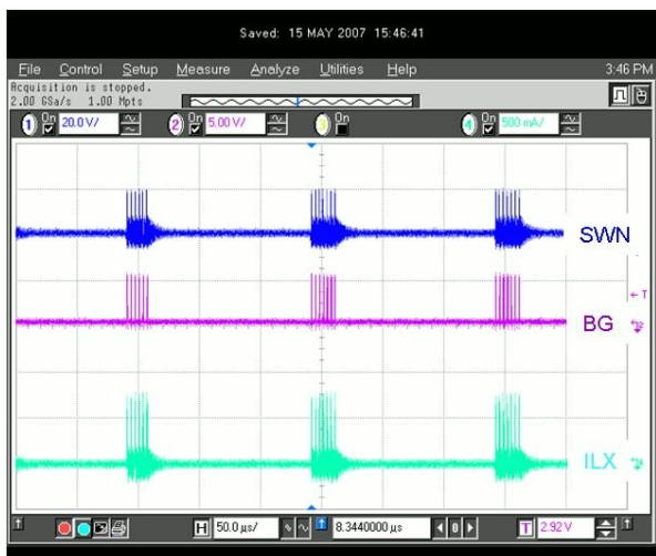
Figure 24. Switcher Operation – Pulse Skipping Mode (PSM)
