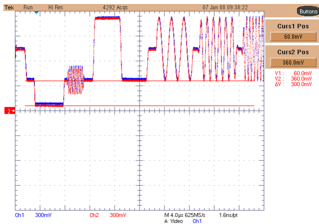
Figure 18. Multiburst Test with Two 150 Ω Loads
