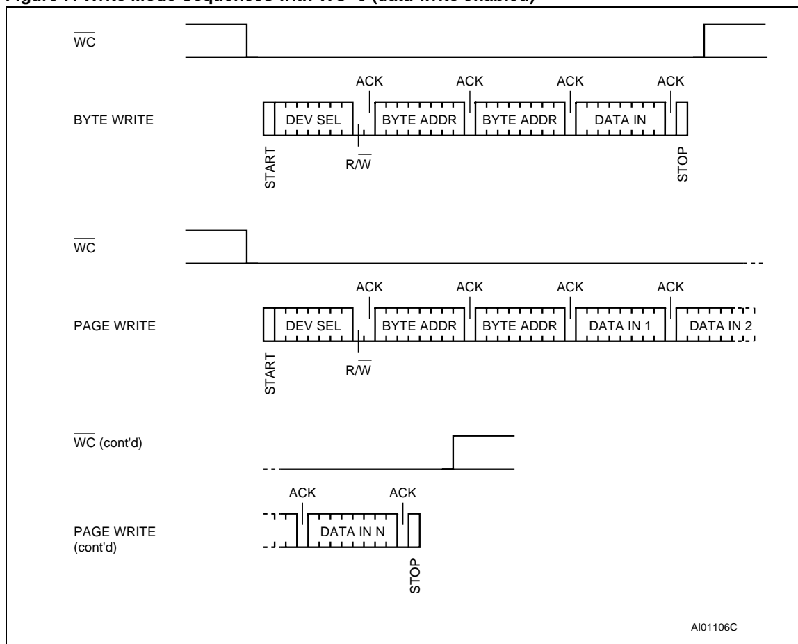
Figure 7. Write Mode Sequences with \overline{WC}=0 (data write enabled)
