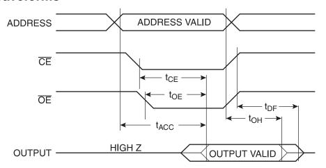
Notes: 1.  $\overline{CE}$  may be delayed up to  $t_{ACC}$  -  $t_{CE}$  after the address transition without impact on  $t_{ACC}$ .
