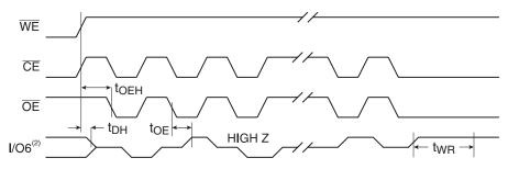
Notes: 1. Toggling either  $\overline{OE}$  or  $\overline{CE}$  or both  $\overline{OE}$  and  $\overline{CE}$  will operate toggle bit.
