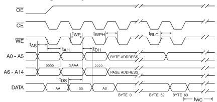
Notes: 1. A0 - A14 must conform to the addressing sequence for the first three bytes as shown above.
