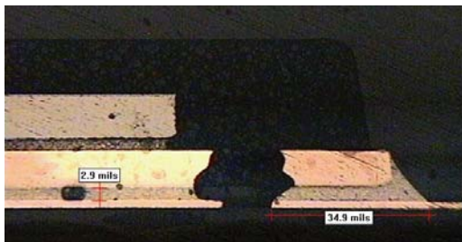
50% Paste Coverage, Plugged Via, 2.9 mil Standoff
