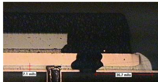
81% Paste Coverage, Encroached Via, 2.1 mil Standoff
