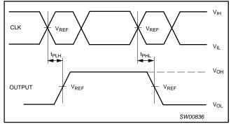
Waveform 1. Propagation delay times
