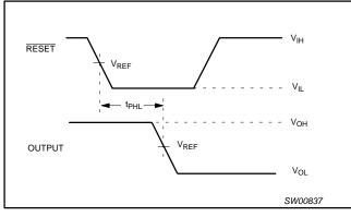
Waveform 2. Propagation delay RESET to output.
