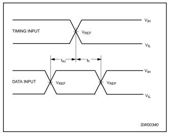
Waveform 4. Setup and hold times
