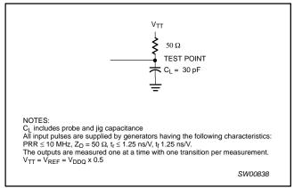
Figure 1. Load circuitry
