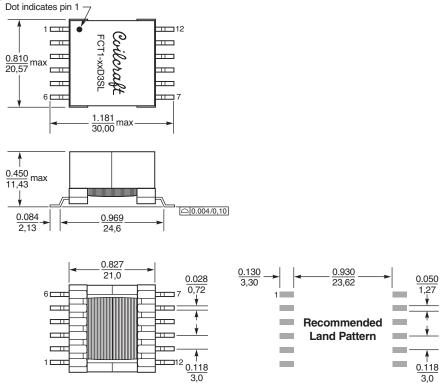
Dimensions are in  $\frac{\text{inches}}{\text{mm}}$
