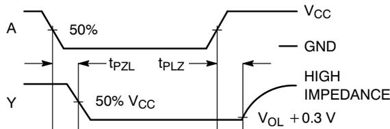
Figure 3. Switching Waveforms
