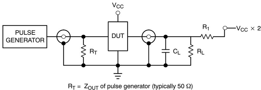
Figure 4. Test Circuit
