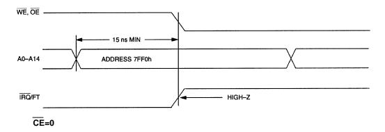
The IRQ/FT pin can also be activated in the battery backed mode. The IRQ/FT will go low if an alarm occurs and both ABE and AE are set. The ABE and AE bits are cleared during the power-up transition, however an alarm generated during power-up will set AF. Therefore the AF bit can be read after system power-up to determine if an alarm was generated during the power-up sequence. Figure 4 illustrates alarm timing during the battery back-up mode and power-up states.
