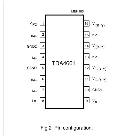
Fig.2 Pin configuration.
