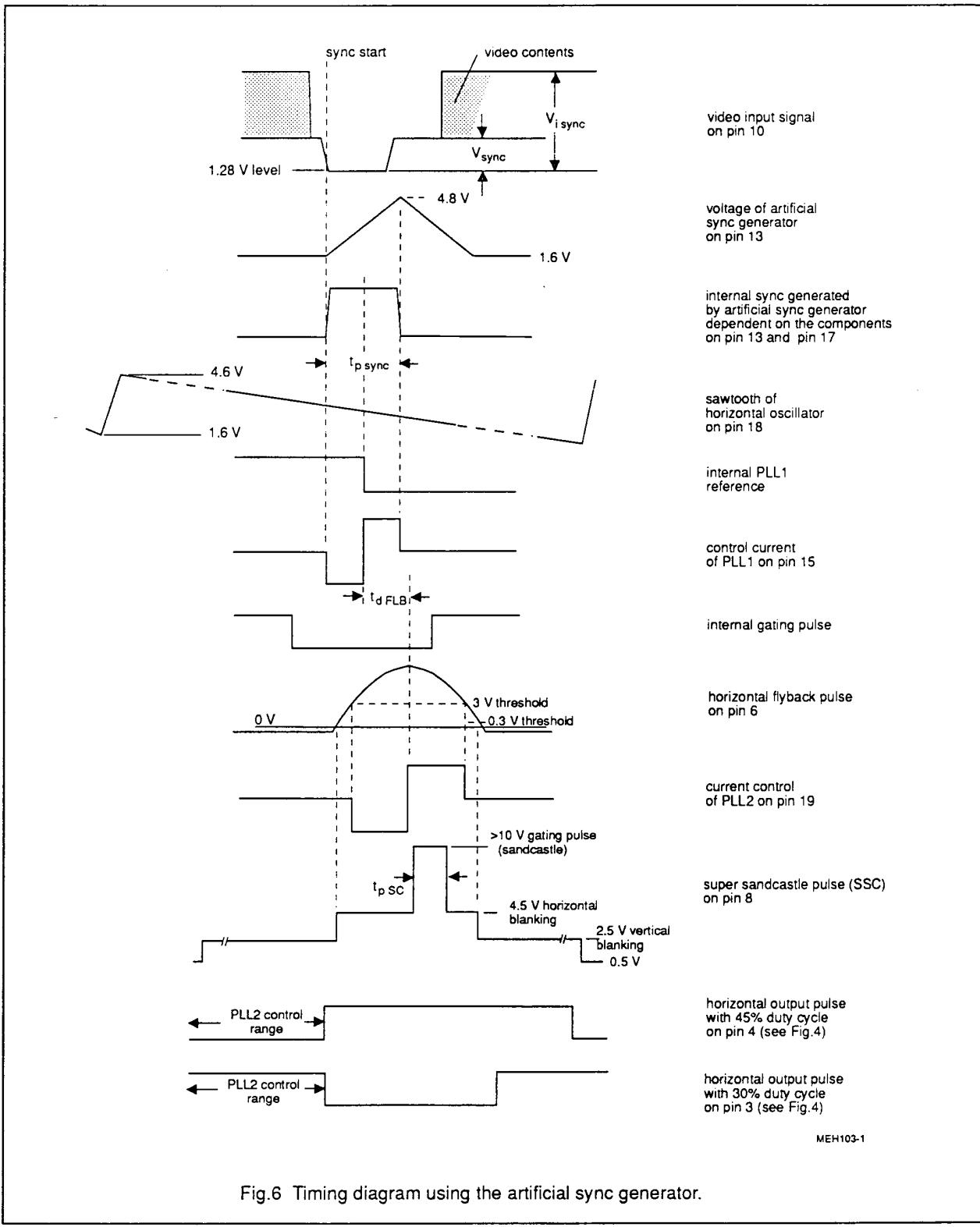
Fig.6 Timing diagram using the artificial sync generator.
