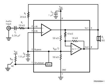
FIGURE 1. Typical Audio Amplifier Application Circuit
