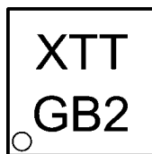
20071302 X - Date Code TT - Die Traceability G - Boomer B2 - LM4923LQ
