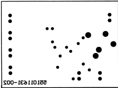
FIGURE 9. Recommended MM PC Board Layout: Bottom-Side Layout
