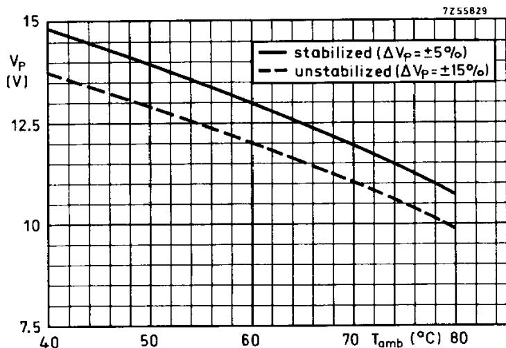
Maximum allowable nominal supply voltage as a function of the maximum ambient temperature.
