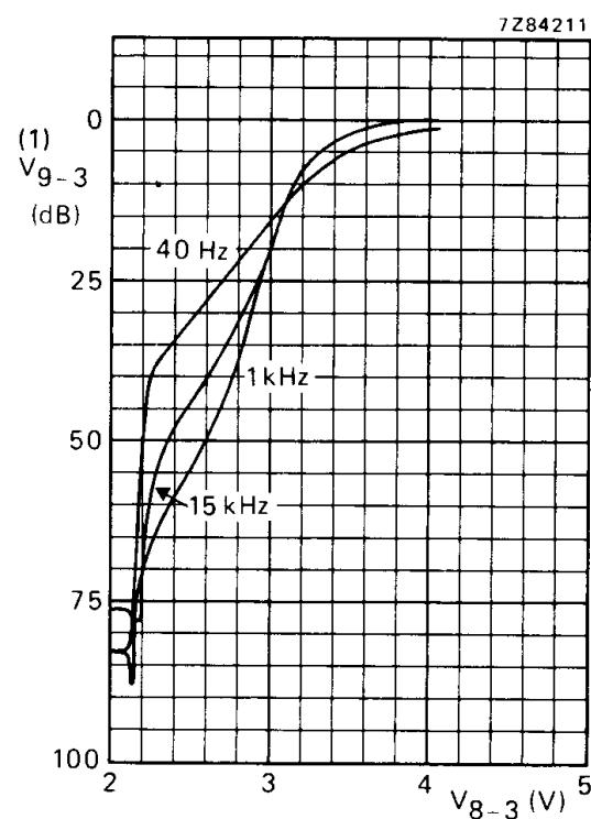
(1) This is actually the a.f. output voltage as shown in Fig. 9.
