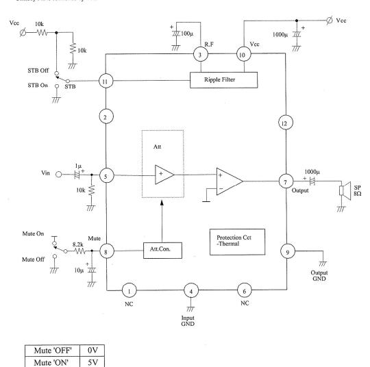
Standby Pin is controlled by Vcc.
