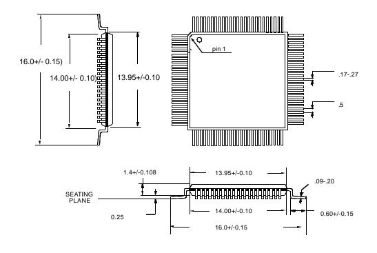
FIGURE 1. 100 pins TP Quad Flat Pack. NS Package Number VJG100A
