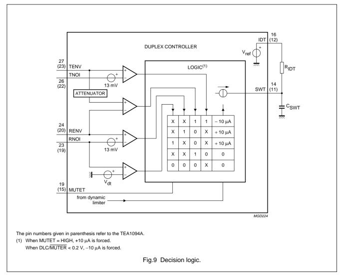
The TEA1094 and TEA1094A select their modes of operation (transmit, receive or idle mode) by comparing the signal and the noise envelopes of both channels. This is executed by the decision logic. The resulting voltage on pin SWT is the input for the voice-switch.
