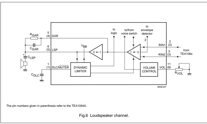
LOUDSPEAKER AMPLIFIER: PINS RIN1, RIN2, GAR AND LSP
