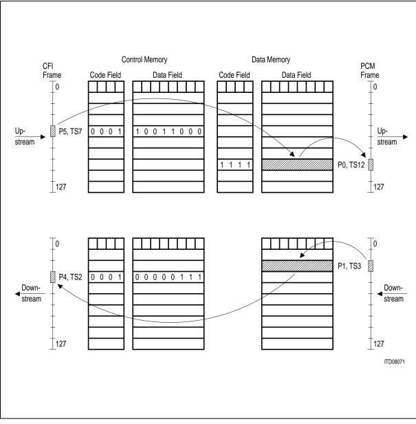
Figure 92 Memory Content of the ELIC<sup>®</sup> for a CFI - PCM Timeslot Connection
