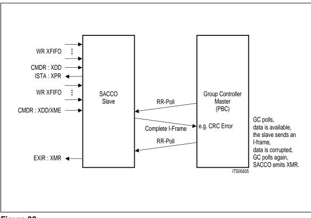
Figure 38 Re-transmission of a Frame
