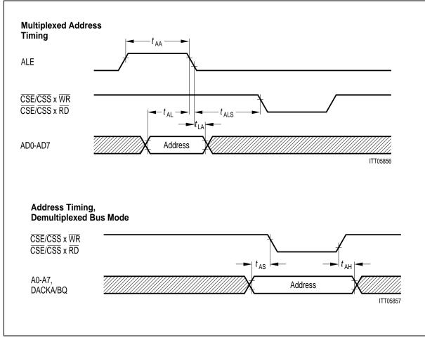
Figure 132 b Siemens/Intel Bus Mode
