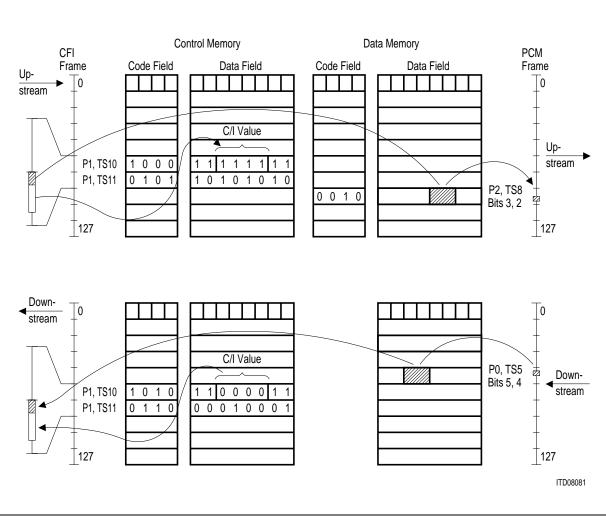
Figure 102 Control Memory Contents for Central D-Channel Handling
