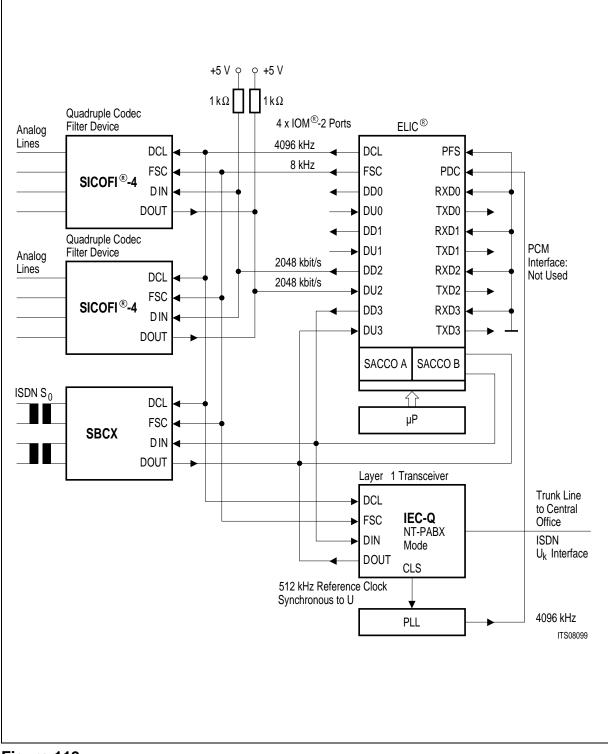
Figure 119 Small PBX with SICOFI®-4, SBCX and IEC-Q
