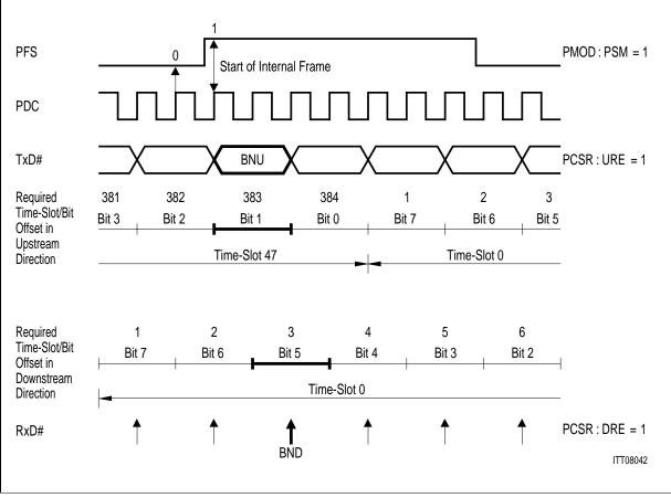
Figure 63 Timing for PCM Frame Offset of Example 2
