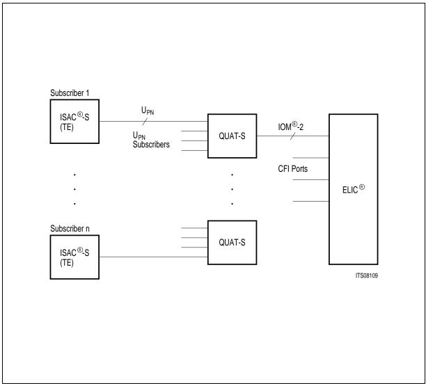
Figure 129 U<sub>PN</sub> Application of ELIC<sup>®</sup>
