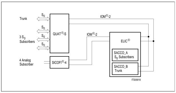
Figure 17 Key System Architecture, Small Size
