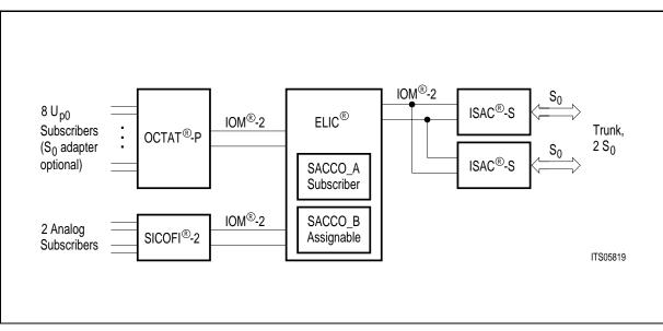
Figure 18 Key System Architecture, Medium Size
