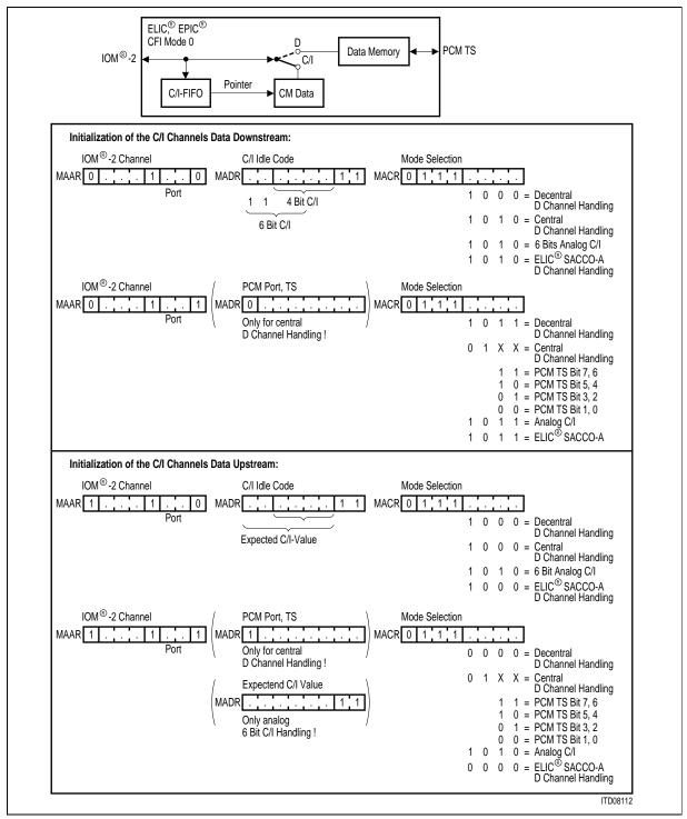
Figure 148 Preparing EPIC<sup>®</sup>s C/I Channels (working sheet)
