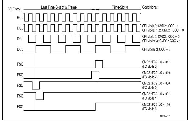
Figure 70 and figure 71 show the position of the FSC pulse relative to the CFI frame:
