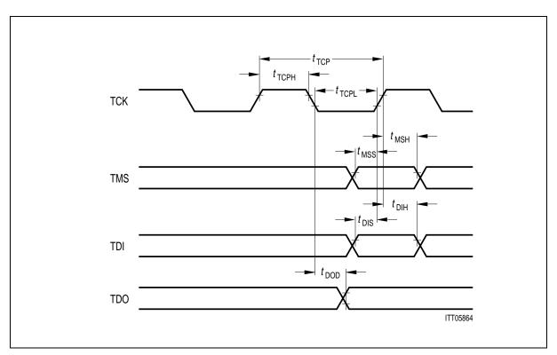
Figure 137 Boundary Scan Timing
