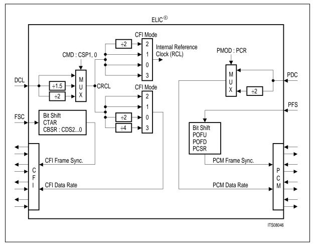
Figure 67 ELIC<sup>®</sup> Clock Sources for the CFI and PCM Interfaces if CMD1:CSS = 1
