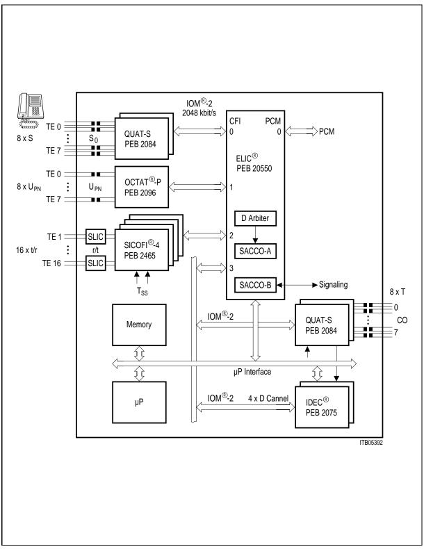
Figure 1 Example for an Integrated Analog / Digital PBX
