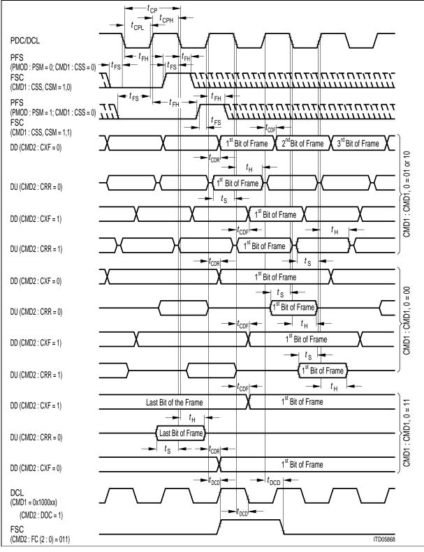
Figure 141 Configurable Interface Timing, CMD:CSP1,0 = 10 (prescalor divisor = 1)
