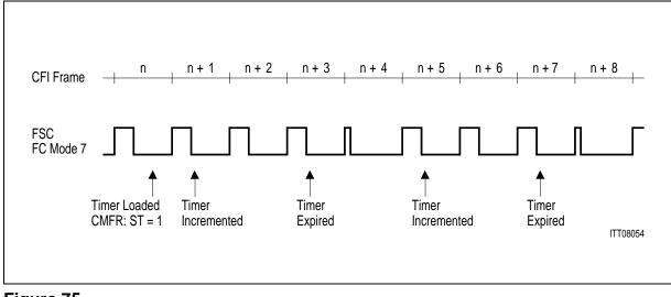
Figure 75 illustrates this behavior for a timer value of TVAL6 ... 0 = 0000001.
