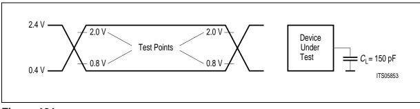
Figure 131 I/O-Wave Form for AC-Test
