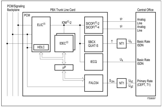
Figure 117 Overview of Trunk Line Applications
