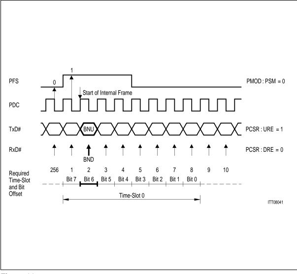
Figure 62 Timing PCM Frame Offset for Example 1
