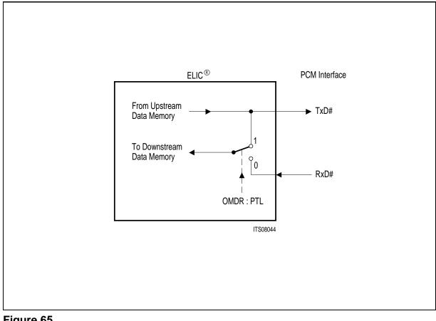
Figure 65 illustrates the effect of the PTL bit:
