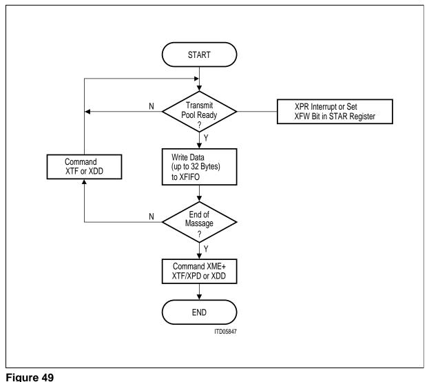
Interrupt Driven Transmission Sequence (flow diagram)
