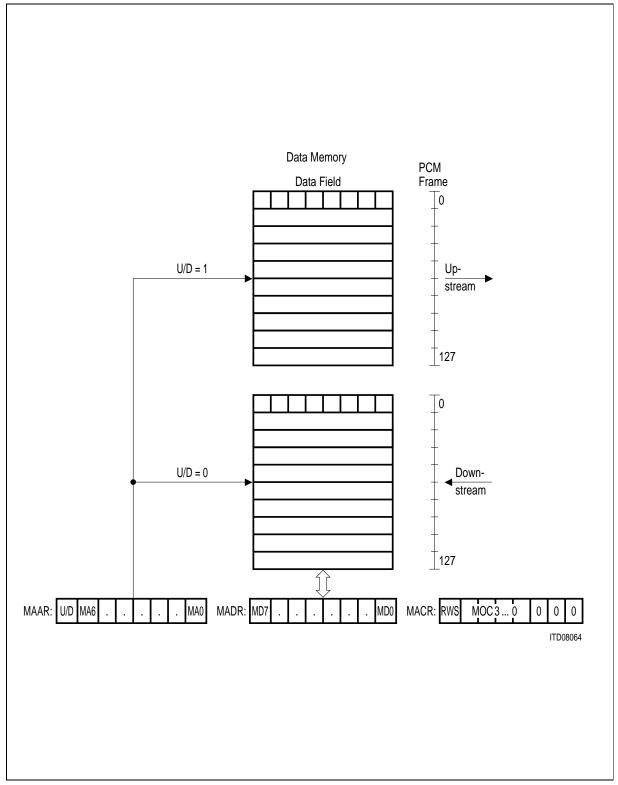
Figure 85 Access to the Data Memory Data Field
