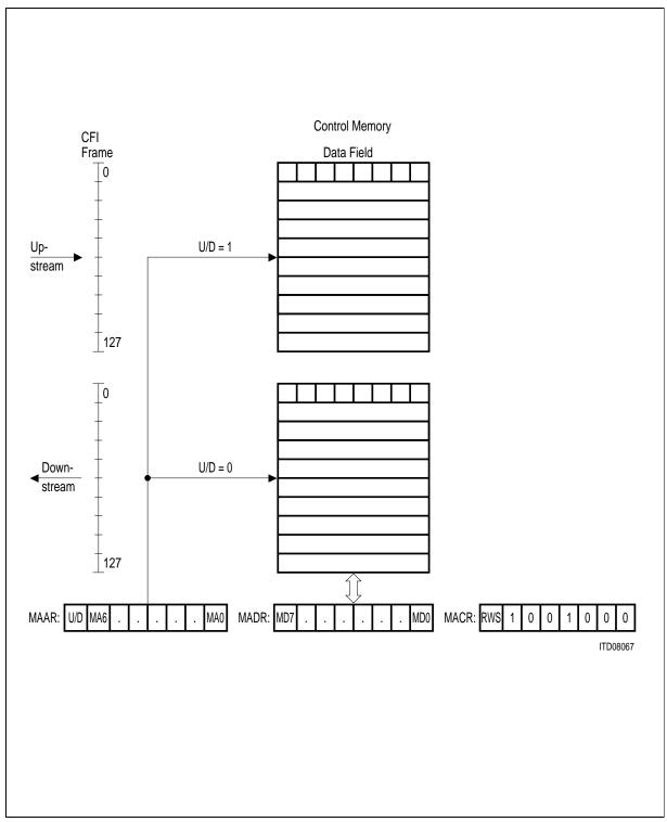
Figure 88 Access to the Control Memory Data Field
