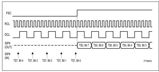
Figure 74 SLD Interface Signals
