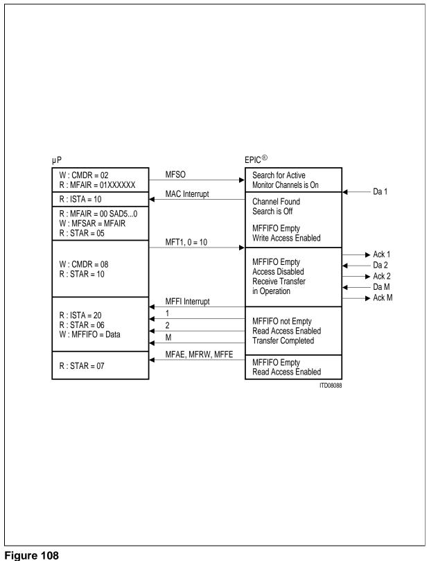
Flow Diagram "Search For Active Monitor Channels Command"
