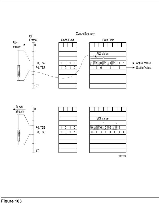
Control Memory Contents for 6-Bit Signaling Channel Handling
