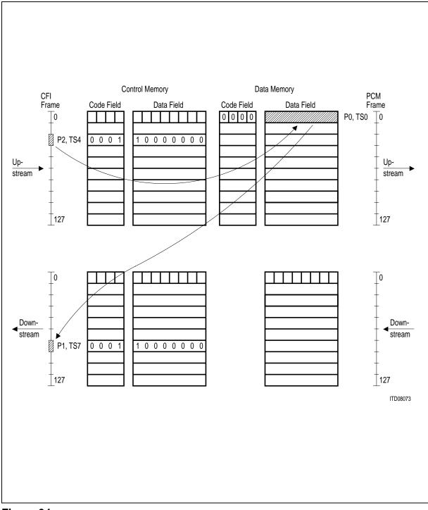
Figure 94 Memory Content in Case of a CFI  $\rightarrow$  CFI Loop
