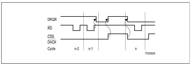
Figure 29 Timing Diagram for DMA-Transfers (slow) Receive (n =  $k \times 32$ )
