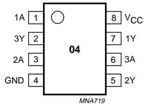
Fig.1 Pin configuration.
