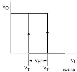
Fig.6 Transfer characteristic.
