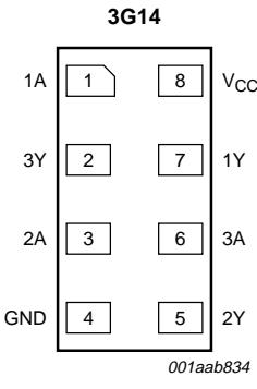
Fig.2 Pin configuration XSON8.
