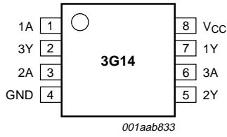
Fig.1 Pin configuration TSSOP8 and VSSOP8.
