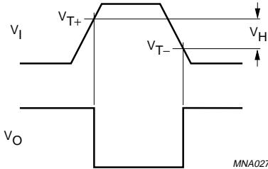
Fig.7 Definitions of  $V_{T+}$ ,  $V_{T-}$  and  $V_H$ .
