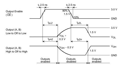
Figure 3  $t_{pLZ}, t_{pHZ}, t_{pZL}, t_{pZH}$
