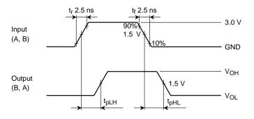
Figure 2  $t_{pLH}, t_{pHL}$
